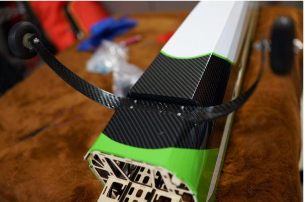
Screw the wheel axles on to the landing gear, and then slide on the wheels and secure in place with the provided grub screws.
