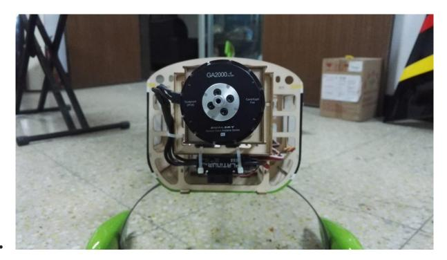
First, locate the secondary firewall box that acts as a standoff for the electric motor. Attach it to the main firewall using the provided bolts and blind nuts.l
