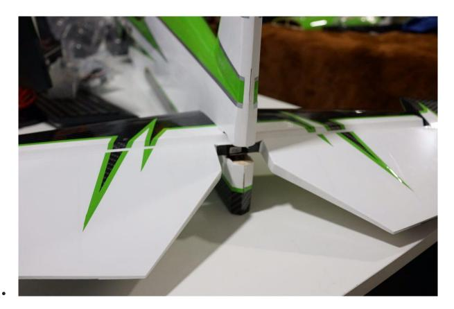
Cut free the trailing edge of the vertical rudder in line with the stabiliser, in order to allow you to slide the stabiliser into the fuselage. Keep the removed section for later.
