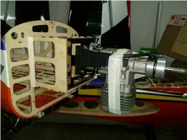
Attach the plastic motor mount to the fuselage, use the mounting screws to secure in place.
