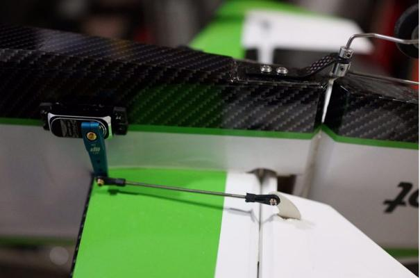
With the model still upside down, position the carbon tail wheel unit on its correct location and mark on the underside of the fuselage to drill the holes for the screws that will hold the tail wheel in place.
