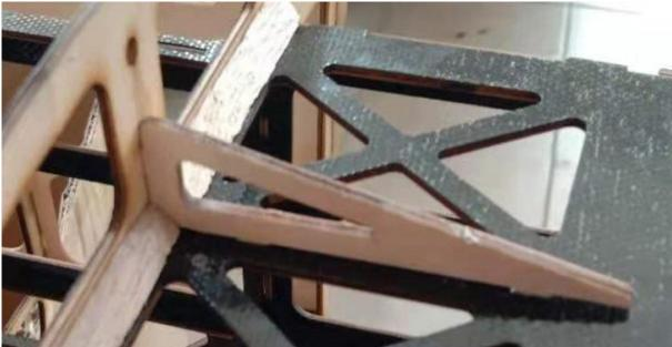
Please note it is important to install the triangular reinforcement for the front former, this helps assure correct alignment between the canopy and the cowl.
