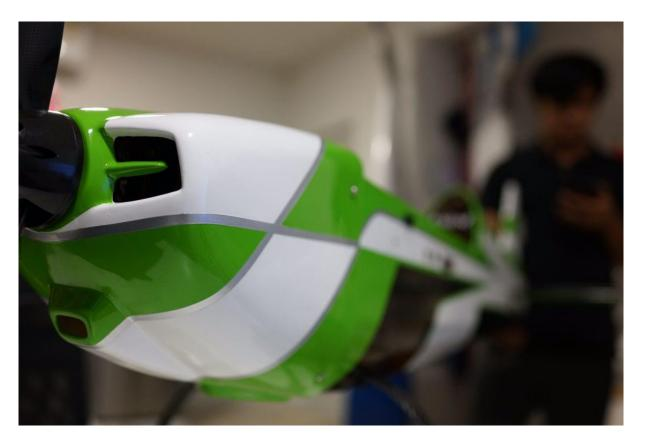
The cowling is installed using four screws that go into four "tabs" in the fuselage.
