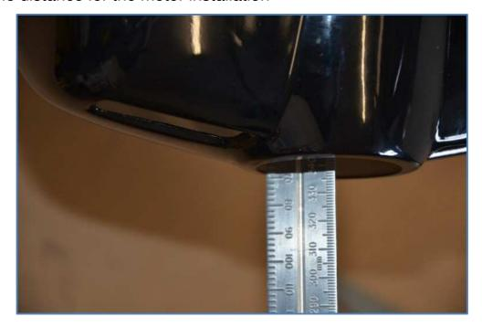
Verification for clearance gap, should be about 1 to 1.5 cm Follow the same procedure for petrol engine
