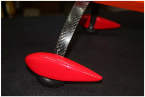
Slide the wheel pants over the wheels and axles, supporting the rear of the pants to line up with the ground and mark where to drill the two screw holes in the wheel pants.
