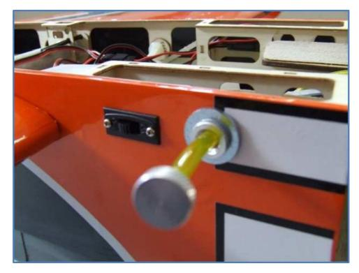
Locate the appropirate hole and install the fuel dot in the side of the fuselage
