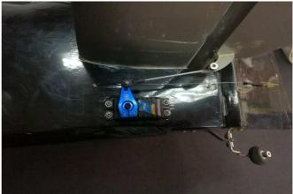
Locate and cut the covering where the servo will be installed, at the rear of the fuselage, under the elevator.
