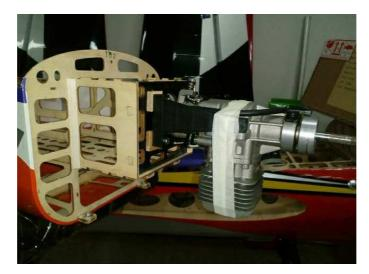
Install the the plastic support to the fuselage, use the mounting screws to tightening it.
