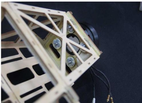
Follow the laser diagram on the firewall to drill the necessary holes for the motor. These are designed for use with the Pilot-RC CC20 motor. If using a different motor, hole position may vary.
