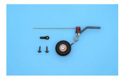
With the model still upside down, position the carbon tail wheel unit on its correct location and mark on the underside of the fuselage to drill the holes for the screws that will hold the tail wheel in place.
