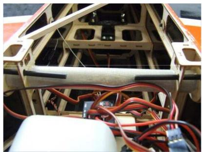
Install the two balance rods in their position as shown in the picture below
