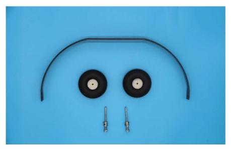
Position the fuselage upside down and screw on the carbon undercarriage to the fuselage using the nuts and bolts provided.
