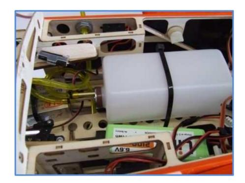
After engine installation, then you can install the engine components like battery, oil tank, receiver, and engine servo(include the servo arm, linkage. ect) in fuselage.
