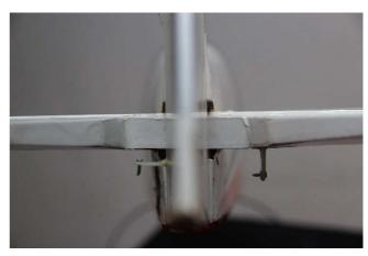
Cut free the trailing edge of the vertical rudder in line with the stabiliser, in order to allow you to slide the stabiliser into the fuselage. Keep the removed section for later.
