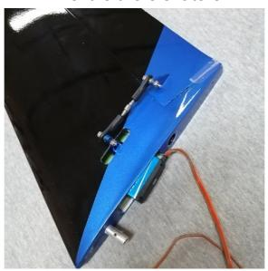
1.Put in the servo to the precut slot in the elevator.
