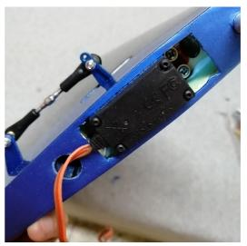
3: The other side of the servo connector glue at the side of the fuselage, just a drop of CA or 5 min epoxy to glue it. After that, use bolt to screw the elevators
