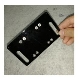
3.Drill out the four holes in the plate, then securely screw the servo to the inside of the plate using the metal screws provided
