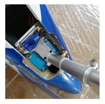
Carefully arrange the nose gear retract wire lead and the steering wire as well ...
