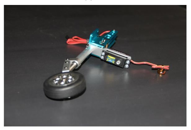
2: Install the servo arm and the push rod. Adjust it to make sure the plane can go straight approx. You still can adjust by radio after install it.
