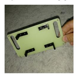
2. Place the servo over the servo plate making sure that the arm moves freely within the provided slot, and mark out the placement of the four screw holes
