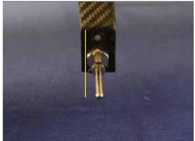
5. Install the collars and wheel in order with a **drop of Blue Loctite** on the collar set screw and ensure the wheel is free to rotate.
