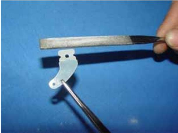
2. Cut out the cover for horns location carefully. Apply the 30 minutes epoxy inside the pre-cut slot, and coat the horn with epoxy
