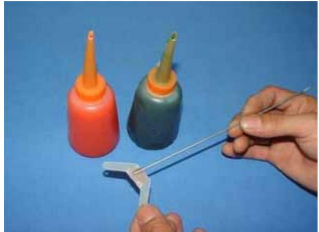
3. Slid the horns into slots slightly. Align the both side before epoxy has cured. Wipe away excess glue with rubbing alcohol
