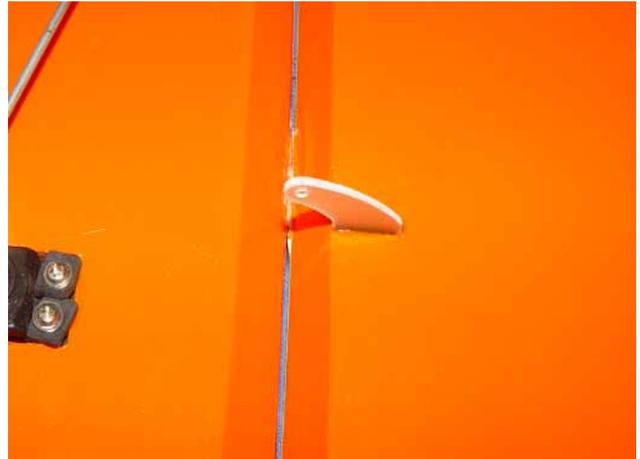
4. Lock the connector with the provided safety clip against vibration and loosened tension as shown
