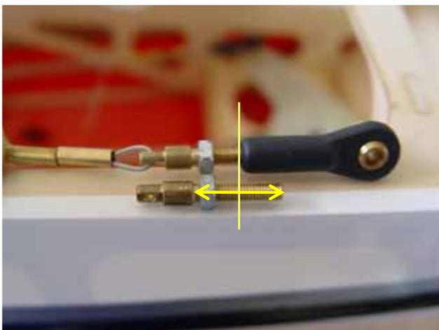
2. Mount servo with mounting screws and face the brand toward the rudder. Install the servo arm ball links with bolts and nuts.
