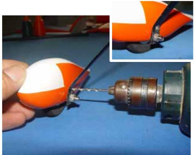
3. Finish the wheel pants mounting with the self-tapping screw
