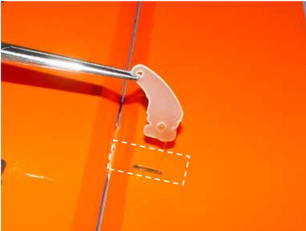
3. Slide the horns into slot slightly and wipe away excess epoxy with rubbing alcohol
