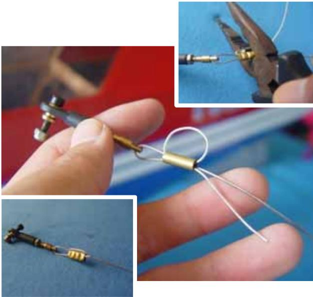
**NOTICE:** The coupler is best to thread half way into ball link for further tightening next
