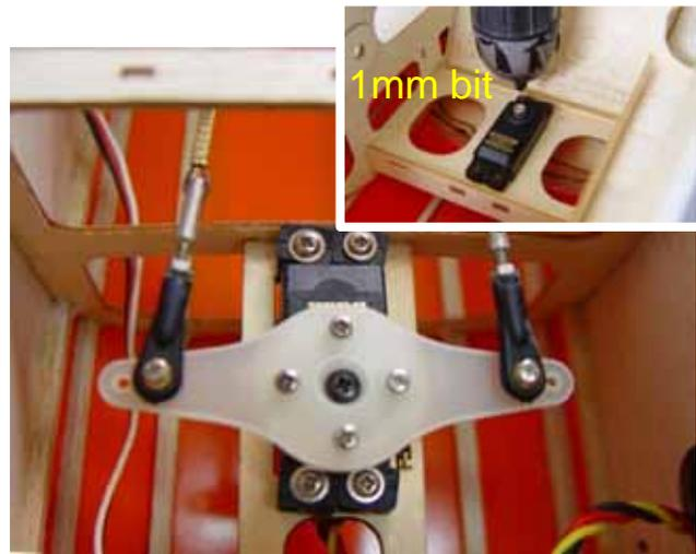
3. The cables are crossover in fuse and threaded out through the rudder horns. **Ensure the same length of cables and tension (Don't pull strongly to hurt the rudder)**
