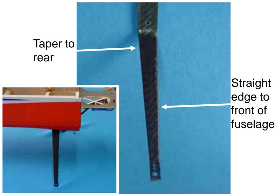
1. Install the landing gear with the bolts. Don't over tighten and crack the carbon fiber
