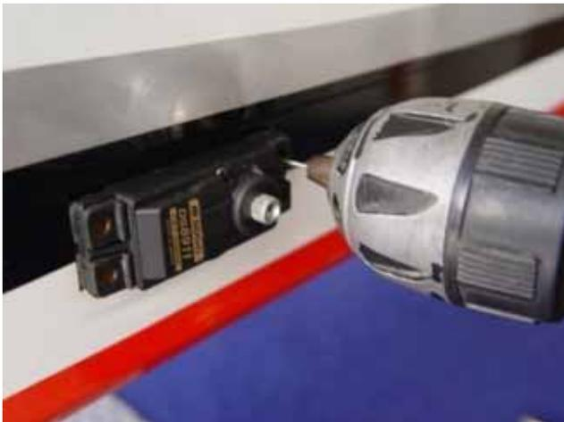
Install the servo arms and measure and cut the extra wire. Then bend to a sharp of "z" as shown. Keep the elevator panel on the neutral position
