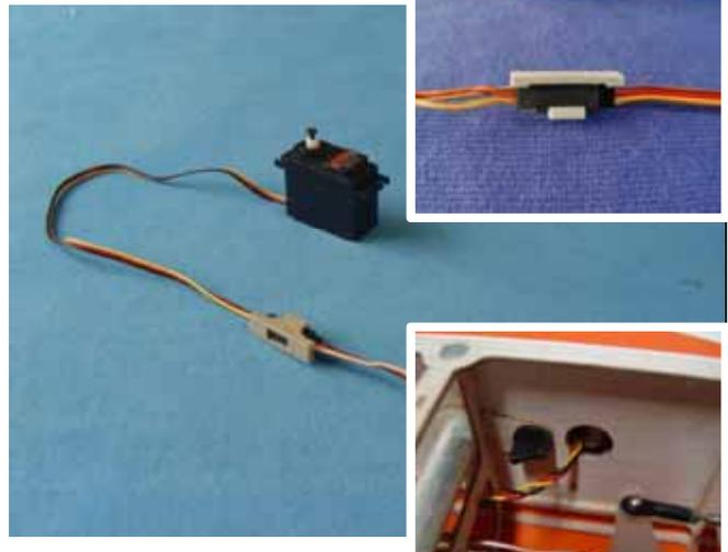
5. Cut out the cover for servo location carefully. Install servo with mounting screws. Use 1mm bit to drill the mounting holes
